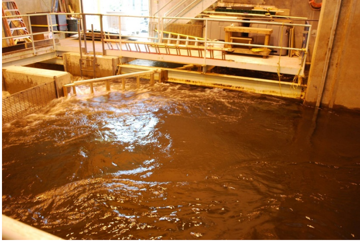
Figure 2. Downstream staging and recovery area. Discharge is toward the left; test flume is out of sight in background, behind the concrete wall to the right. The screen continues to arc toward the back wall as shown in Figure 1a. Note the slack water condition, which provided suitable resting conditions for both Atlantic salmon and American shad.
