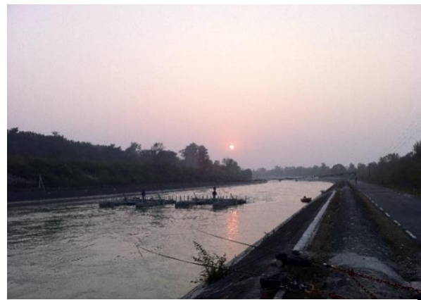
Fig. 5 Two 25kW units operating on the Chilla Canal in Northern India
