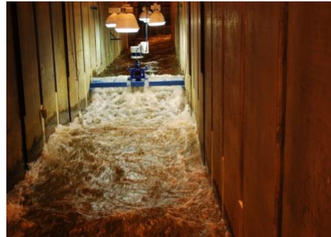
Fig.3 EnviroGen turbine installed and operating in the test flume where fish were released and monitored.
